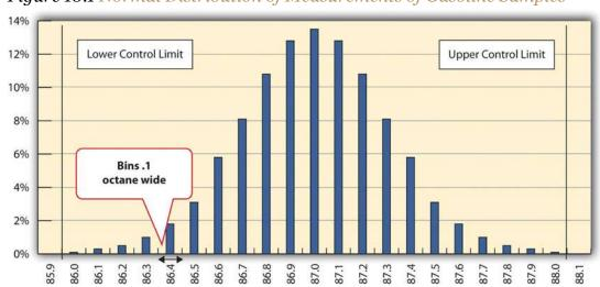
Figure 10.1 Normal Distribution of Measurements of Gasoline Samples
